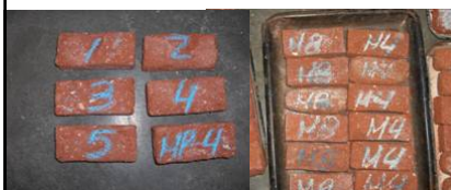
T: 1000 C, 4 h burning, control series (right) and sample made with 5% calcium carbonate
