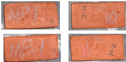
T: 900 C, 3 h burning, control series (right) and sample made with 5% calcium carbonate
