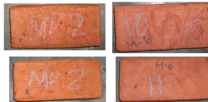
T: 900 C, 4 h burning, control series (right) and sample made with 5% calcium carbonate
