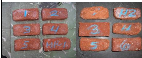
T: 900 C, 3 h burning, control series (right) and sample made with 5% calcium carbonate
