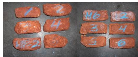
T: 900 C, 4 h burning, control series (right) and sample made with 5% calcium carbonate
