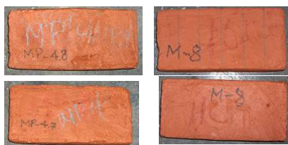
T: 1000 C, 3 h burning, control series (right) and sample made with 5% calcium carbonate
