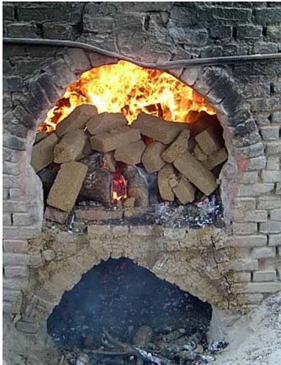
Firing a batch kiln with Solid Fuel Briquettes
