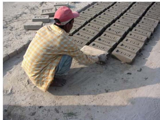
Sand molding clay bricks
