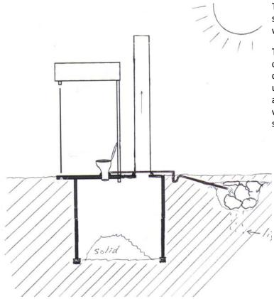
The degradation toilet is a a version of the Otji toilet system recommended for very remote areas and where maintenance causes problems.
